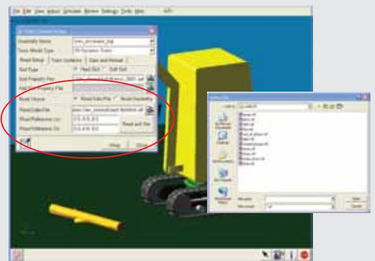
**Automatically wrap track segments around the wheels**
