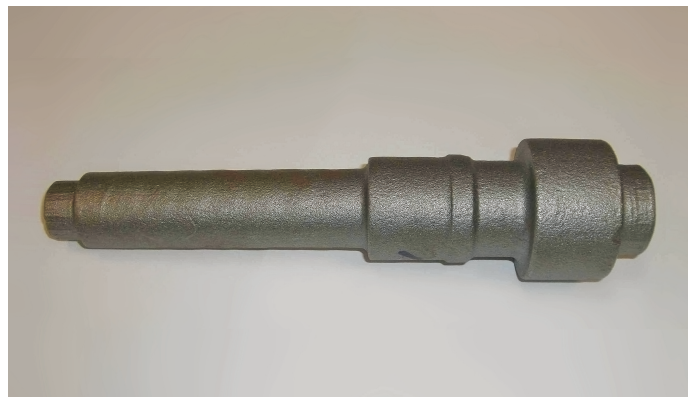
After Inductive Heating to 1240 Degrees, the Component Is Formed on a Cross Wedge Roll
